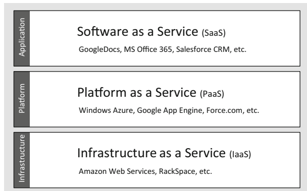
Fig. 1 Cloud computing architecture layers
